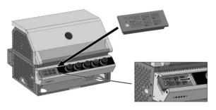
Step 4. Attach the bracket to lock the digital display panel. Use the two screws from Step 1.
