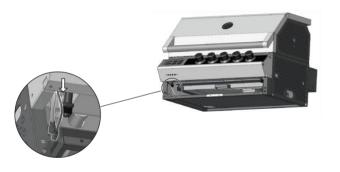
b. Slide in the digital display panel into place in the cavity.
