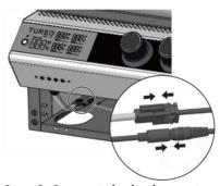
Step 6. Connect the barbeque transformer to the power supply.
